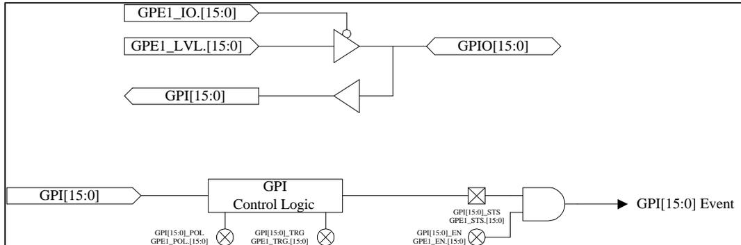
Figure 21.2-3 Hardware Model for Generic Feature 1 (GPE1)
