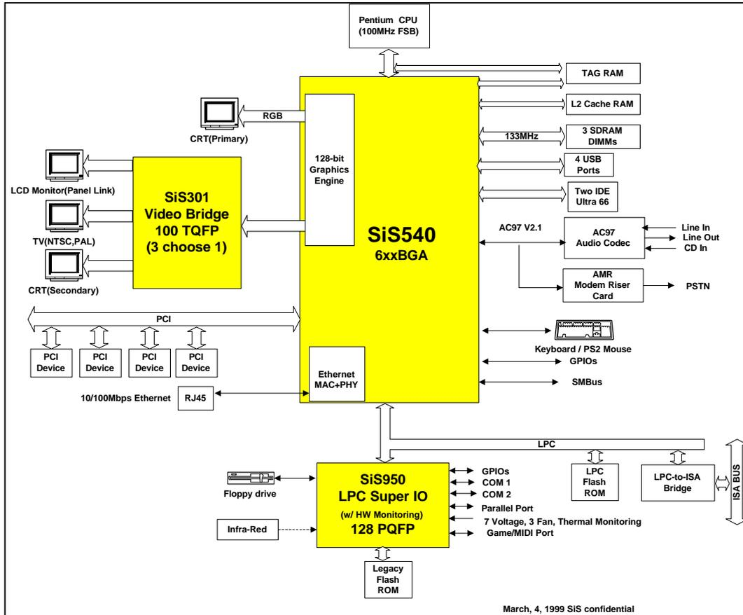
Figure 1-1 SiS540 System Block Diagram
