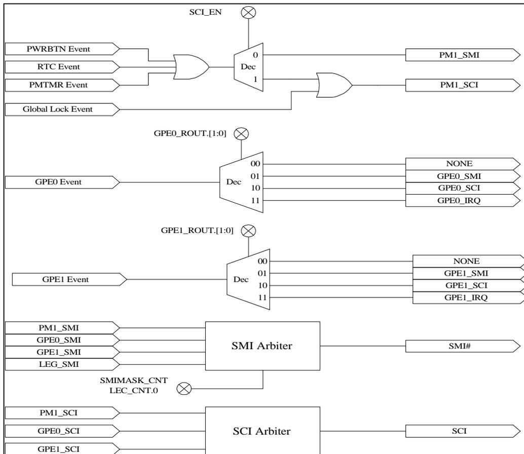
Figure 21.3-1 Interrupt Model for ACPI
