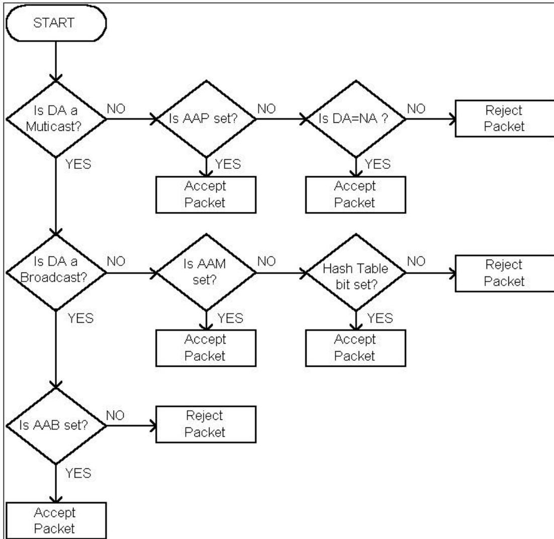
**Figure 13.3-1 Receive Filter Algorithm**
