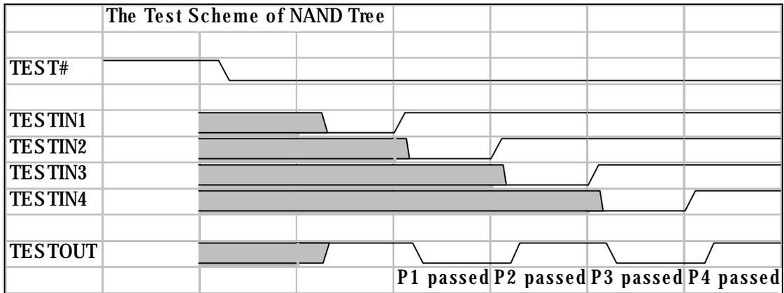
Figure 6.8-2 The Test Scheme of NAND Tree
