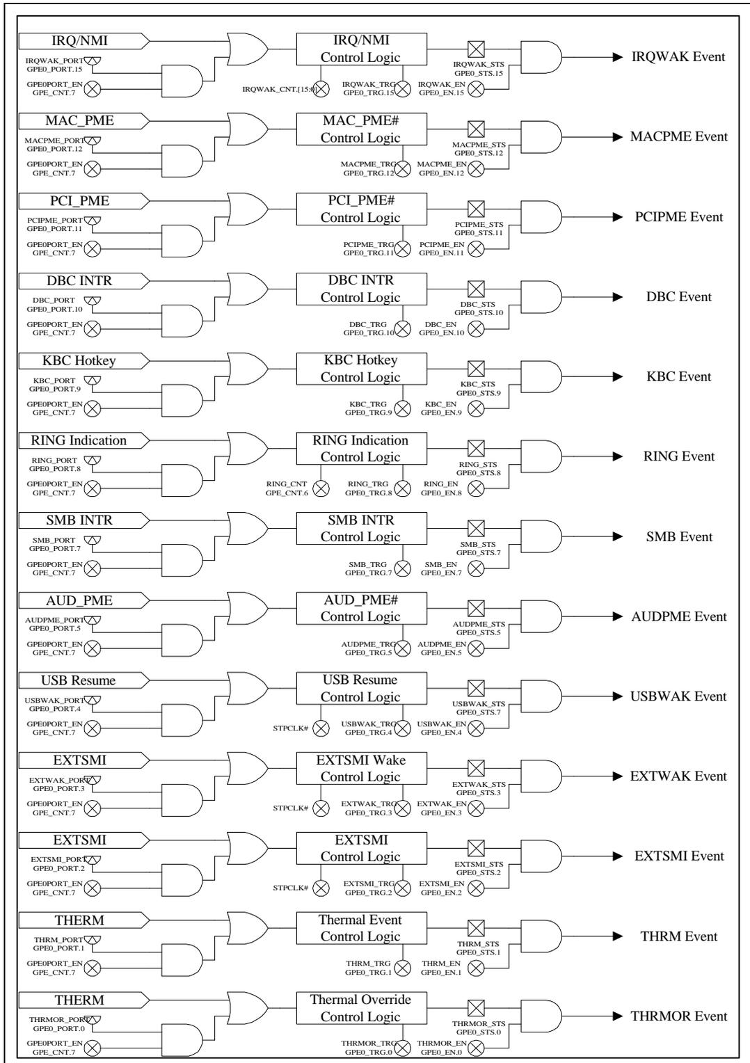
**Figure 21.2-2 Hardware Model for Generic Fixture 0 (GPE0)**
