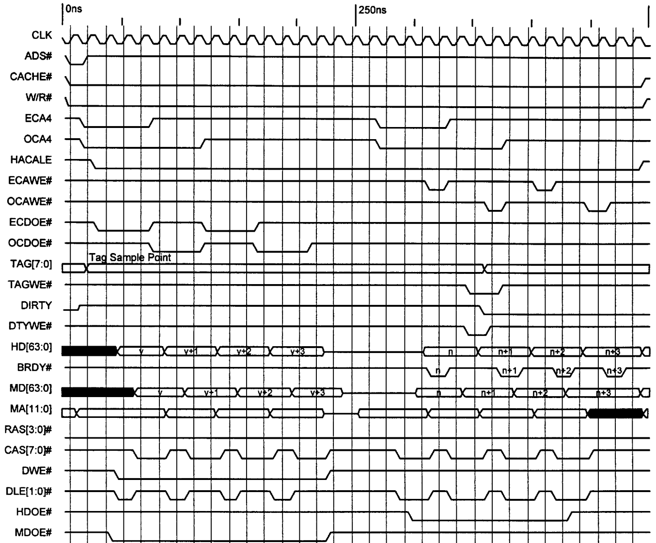
Figure 4-12 L2 Cache Read Miss Dirty Cycle - Async. SRAMs
