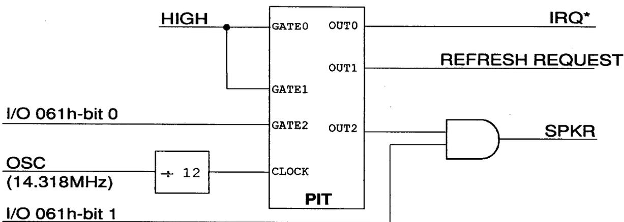
**Figure 19 - HT25 Programmable Interval Timer**
