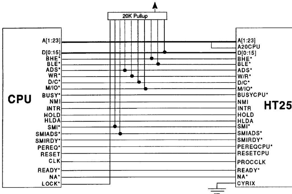
Figure 3a - HT25 AM386™ SXLV CPU Interface
