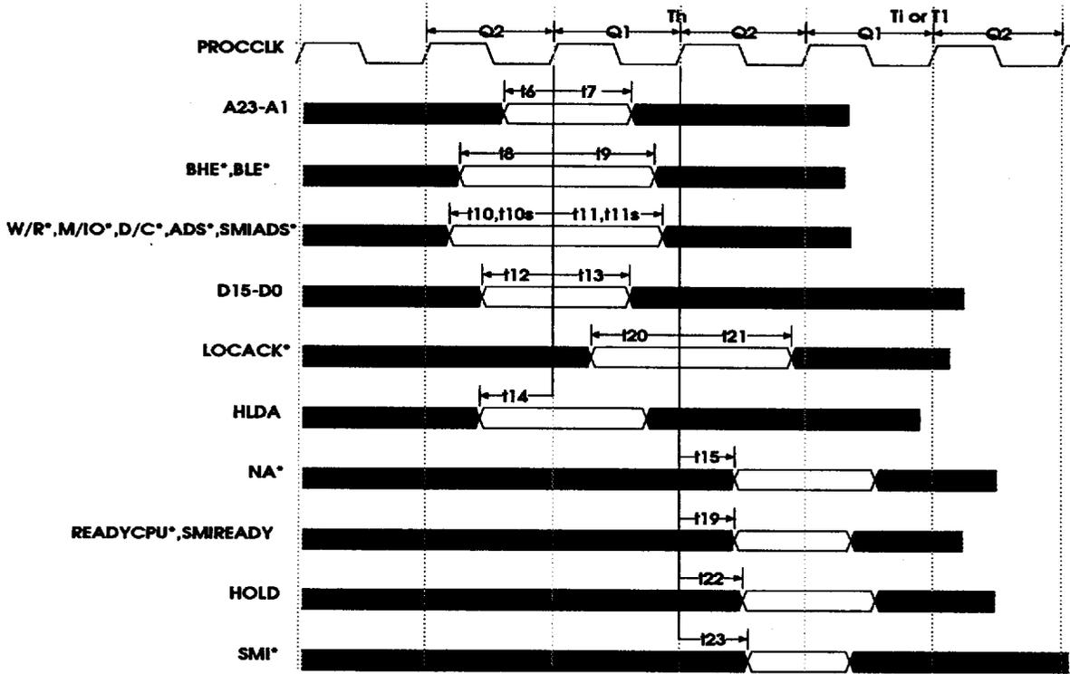
**HT25****3V Single Chip 386SX Controller****AC Specifications****ISA Bus Timing**
