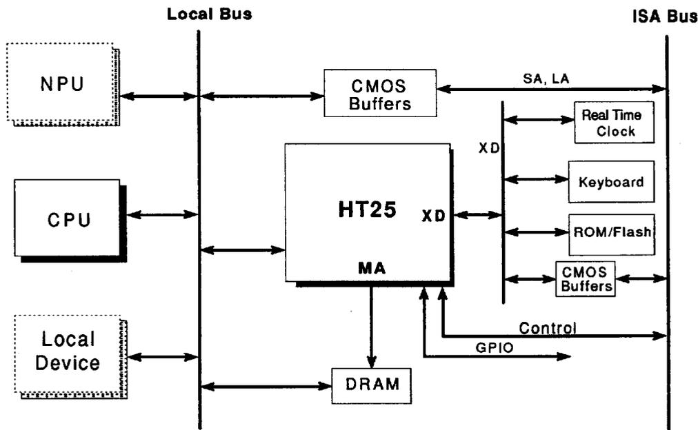
Figure 1 - HT25 Based System Implementation
