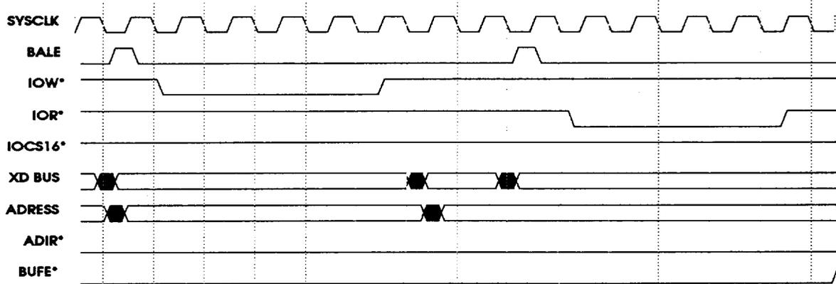
Figure 12a - ISA 8 Bit I/O Cycle
