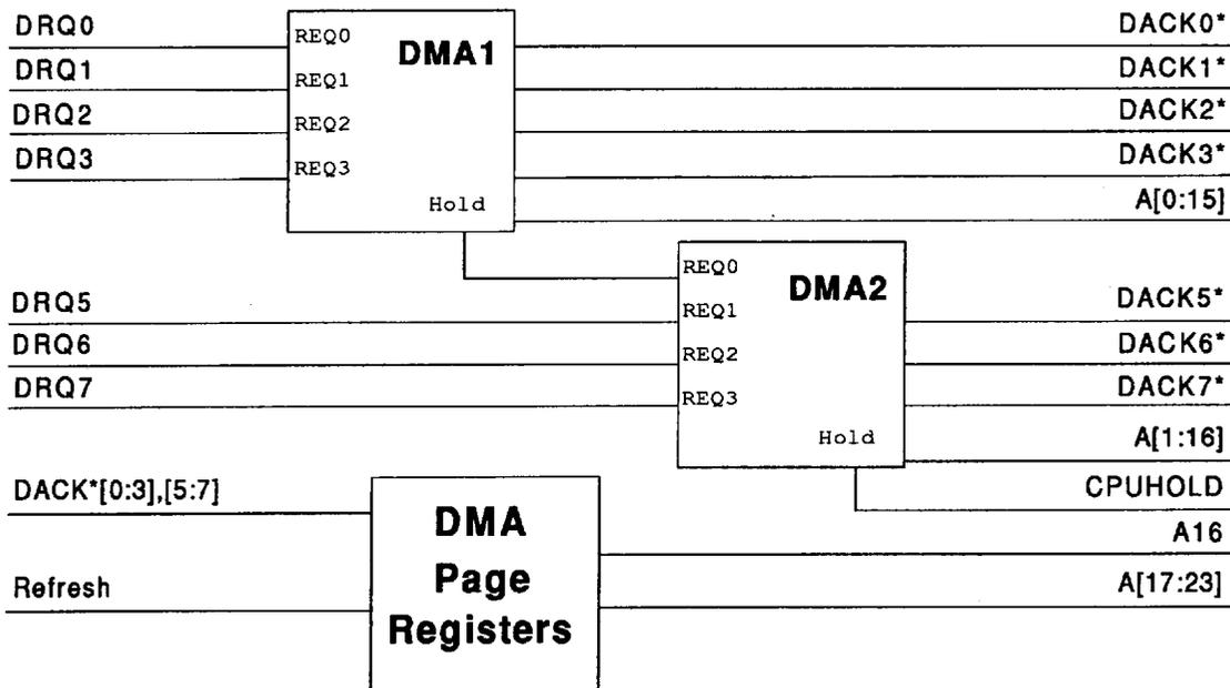
**Figure 16 - HT25 DMA Controller**
