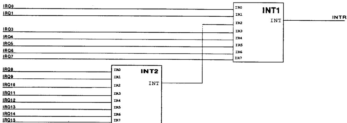
**Figure 18 - HT25 Interrupt Controller**
