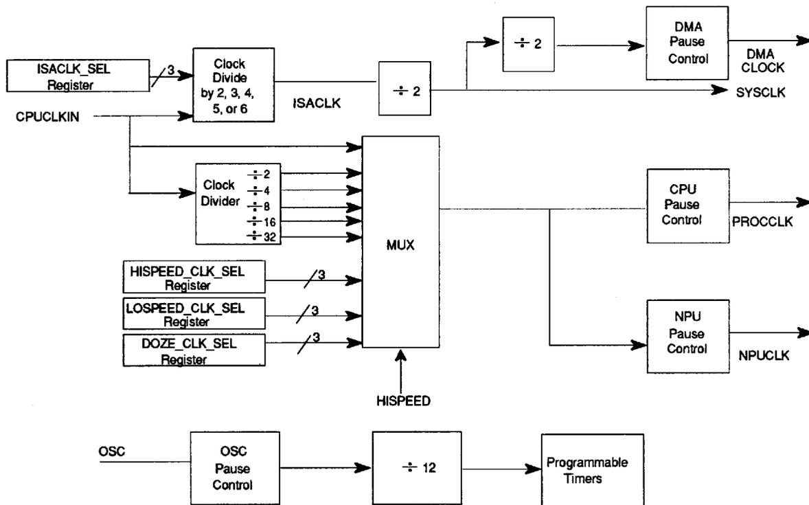
**Figure 4 - Clock Control Diagram**
