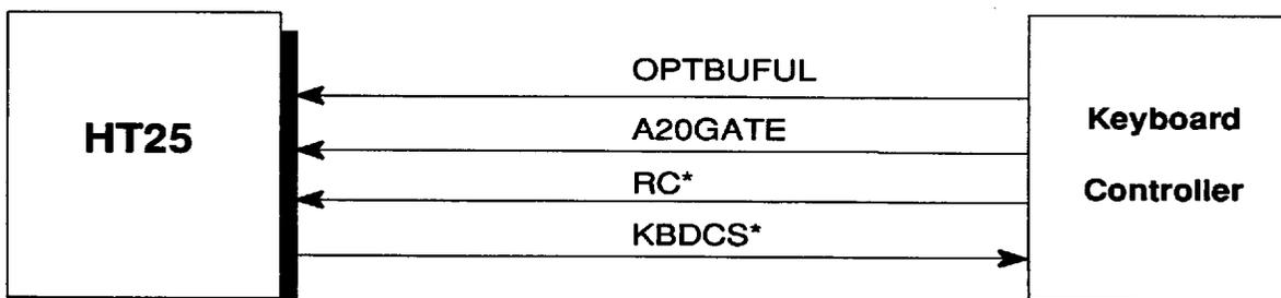
Figure 15 - Keyboard Controller Interface
