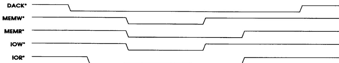
**Figure 17 - DMA Functional Timing**
