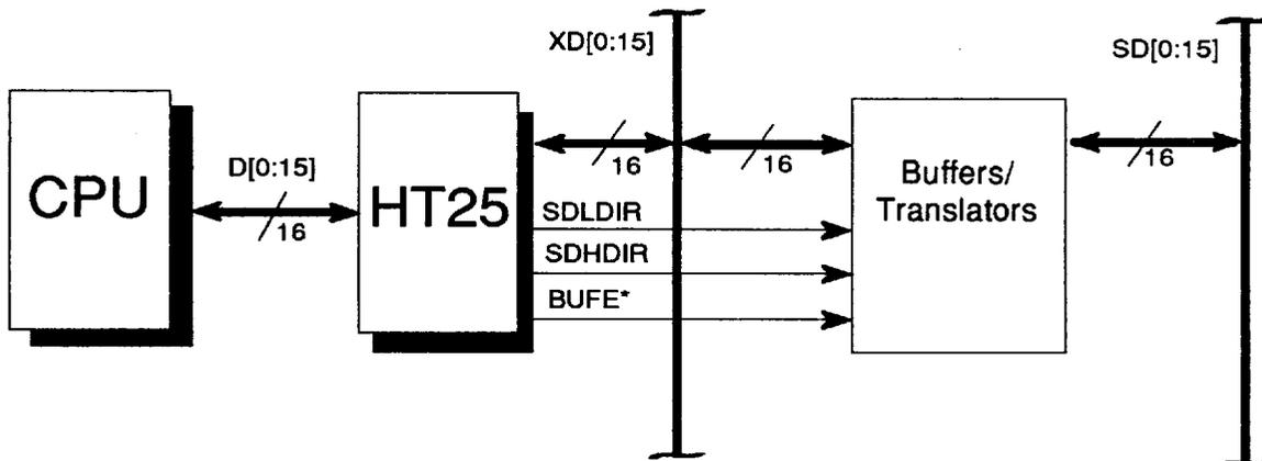
Figure 11 - XD and SD data bus architecture.
