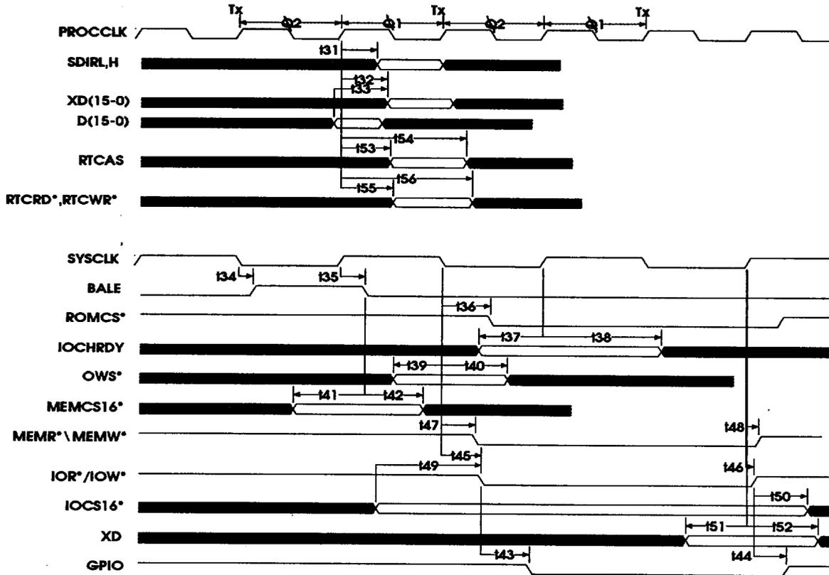
**HT25****3V Single Chip 386SX Controller****AC Specifications****DMA Timing**
