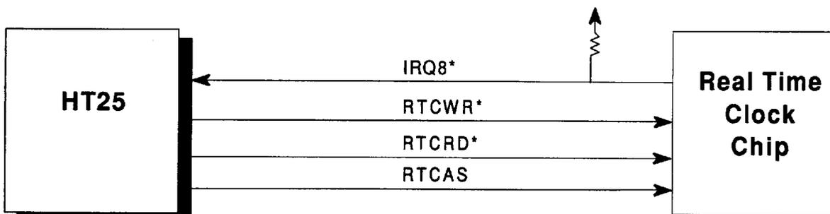
Figure 14 - Real Time Clock Interface
