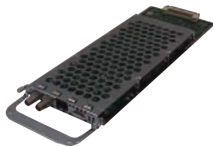
Figure 2 CT3 Termination Card
